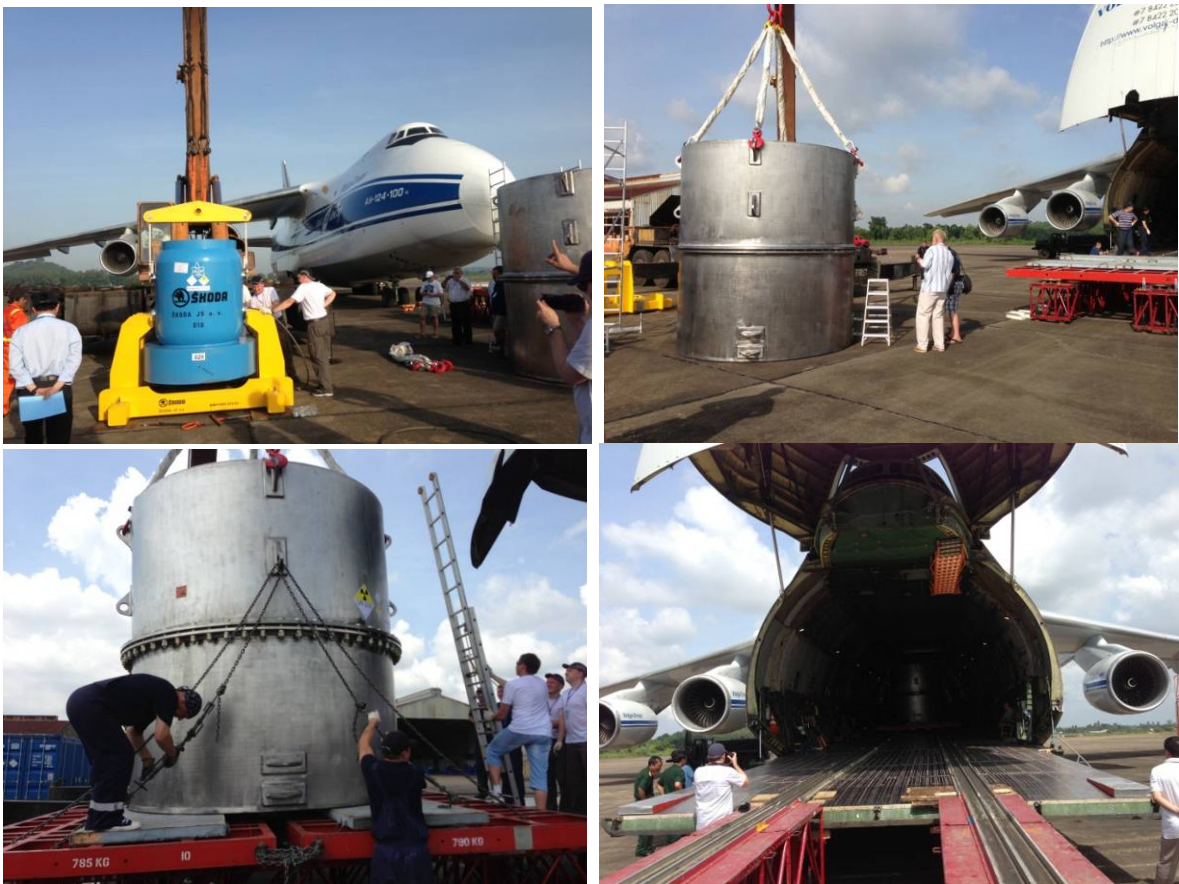
Fig. 10. Building up the TUK-145/C package and loading it into the aircraft
