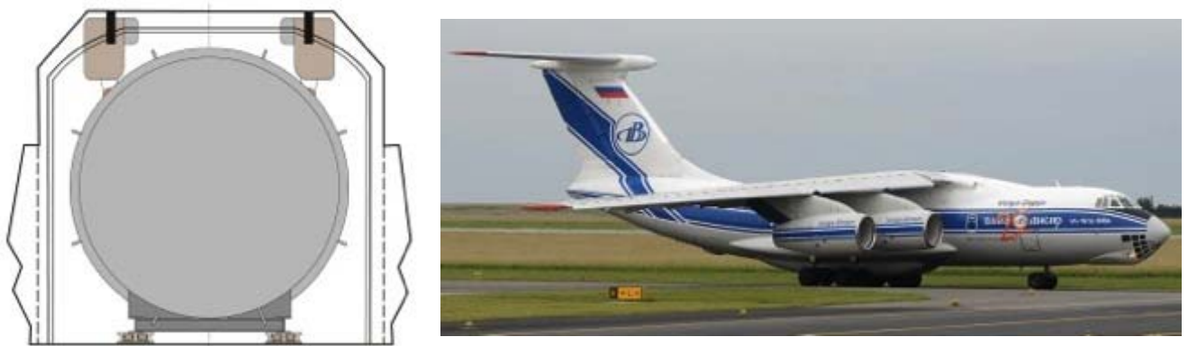
Fig.6. TUK-145/C loading in the IL-76 aircraft using the special handling frame (Option 3)
