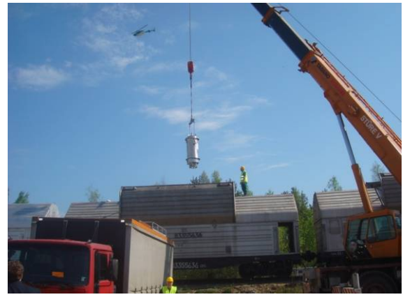
Fig. 1. Installing the TUK-19 casks onto a truck (a) and into a TK-5 rail car (b)
