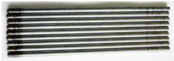
FIG. 5. Simulators of non-oxidized fragments of fuel rod claddings.
