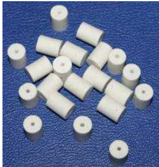
FIG. 2. Simulators of fuel pellets from electro-technical casting porcelain.
