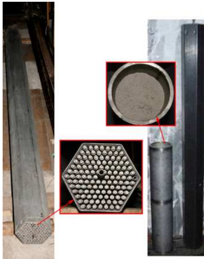
FIG. 8. Simulators of SNF for canister 28.
