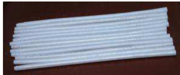
FIG. 6. Simulators of oxidized fragments of fuel rod claddings.
