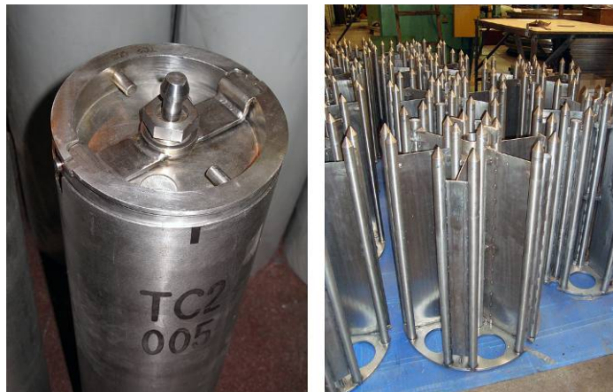
Fig.2. Untight canisters with SNF and baskets for the SKODA VPVR/M cask
