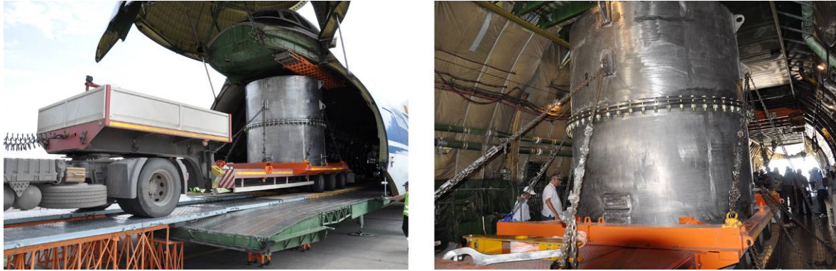
Fig. 5. Loading a truck with the TUK-145/C packaging into AN-124-100 aircraft
