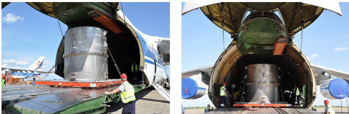
Fig. 4. Loading the TUK-145/C packaging into AN-124-100 using a roller system
