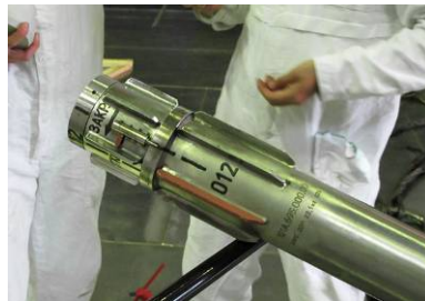
Fig.7. Canister for transportation of fuel rod bundles of non-conforming RBMK SFAs
