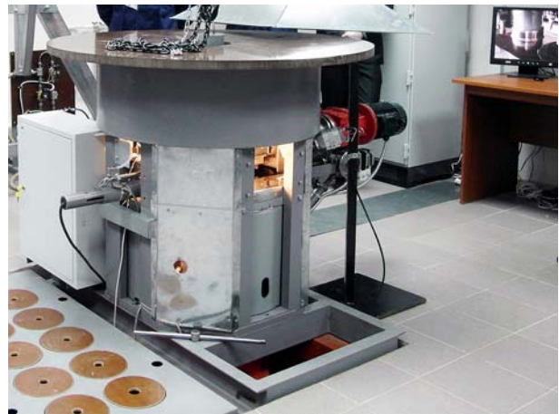
Fig. 3. Prototype facility for cutting canisters and SFA encapsulation
