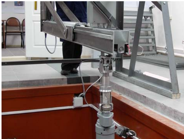
Fig. 2. Prototype manipulator for removal of the SFA canisters from the storage pool
