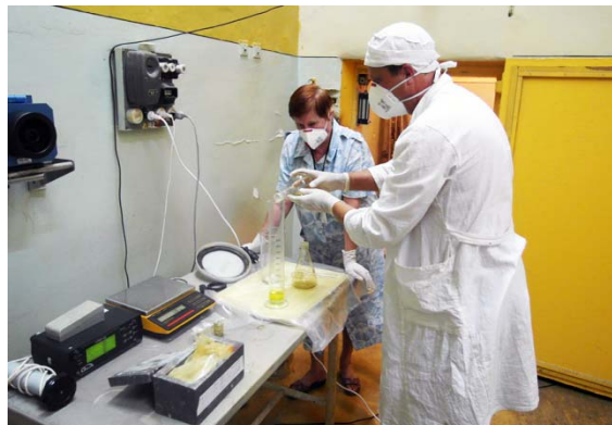
Fig. 3. Measuring the volume of the fuel samples taken in the isotope storage room
