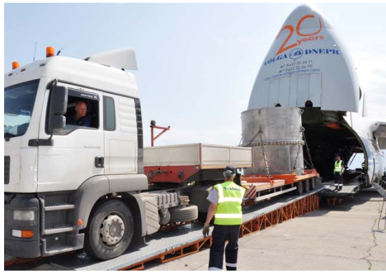
Fig. 4. Loading TUK-145/C package installed on a truck into AN-124-100 Ruslan aircraft
