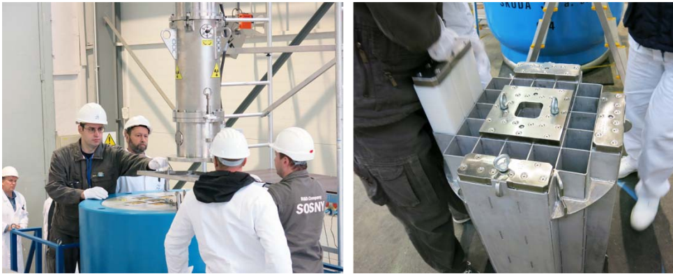
Fig. 7. Dry Run of equipment to verify its compatibility with SKODA VPVR/M cask
