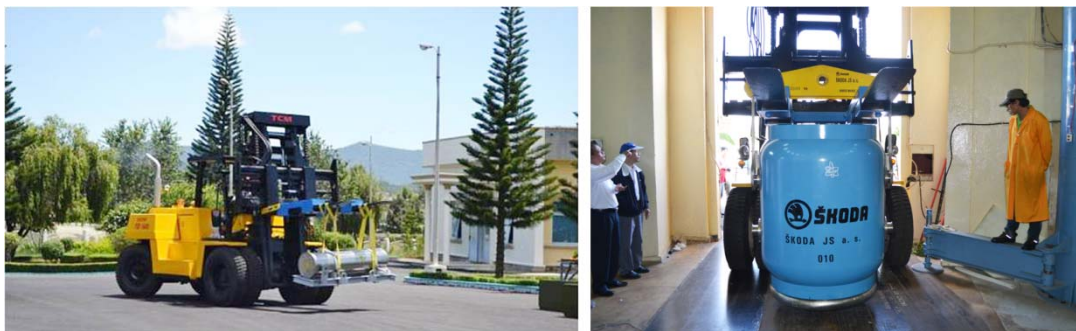
Fig. 1. Unloading of Equipment and Delivery of SKODA VPVR/M Cask to Reactor Hall with a Forklift
