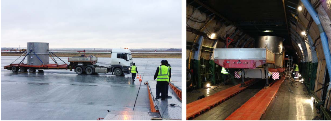
Fig. 7. Delivery of TYK-145/C Package to Airport and Its Fastening in AN-124-100 Aircraft
