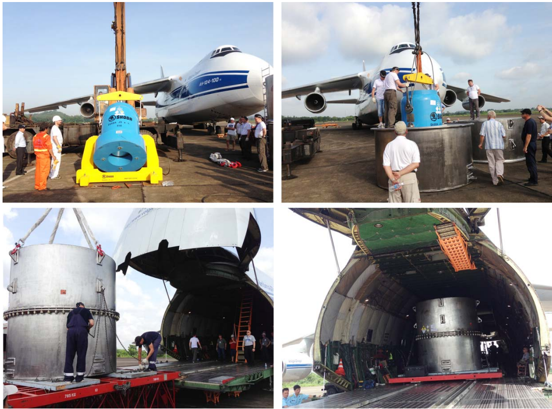
Fig. 4. Buildup of TUK-145/C Package and Loading into AN-124-100 Plane
