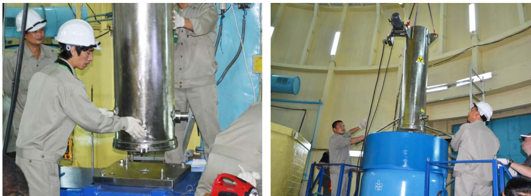
Fig. 3. Unloading of SFAs from Storage Pool and Loading into SKODA VPVR/M cask Using Transfer Cask
