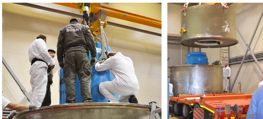
Fig. 6. Build-up of TYK-145/C Package on Semi-Trailer
