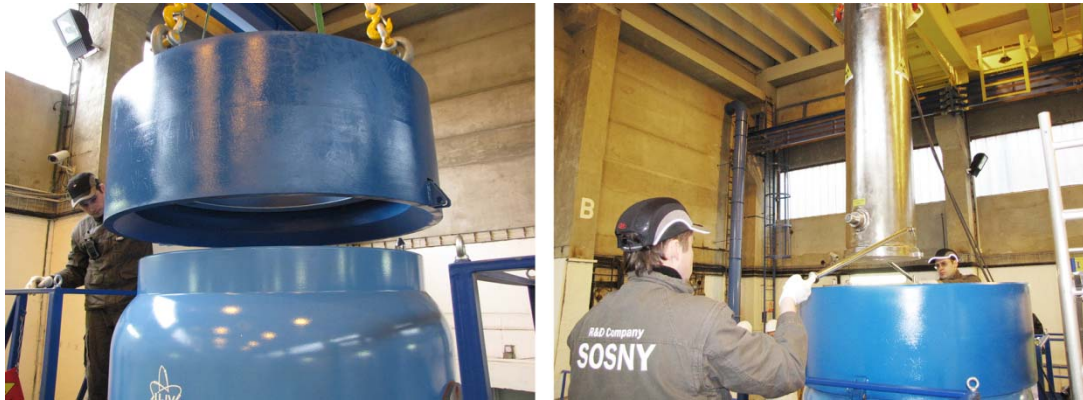
Fig. 2. Dry Run of Newly Developed Equipment to Verify Its Compatibility with SKODA VPVR/M Cask
