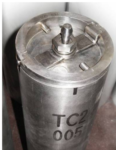
Fig. 1. Non-tight canister for damaged spent fuel shipment
