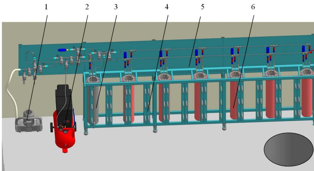
1 – vacuum pump; 2 – compressor; 3 – dosator; 4 – rack; 5 – stand;
