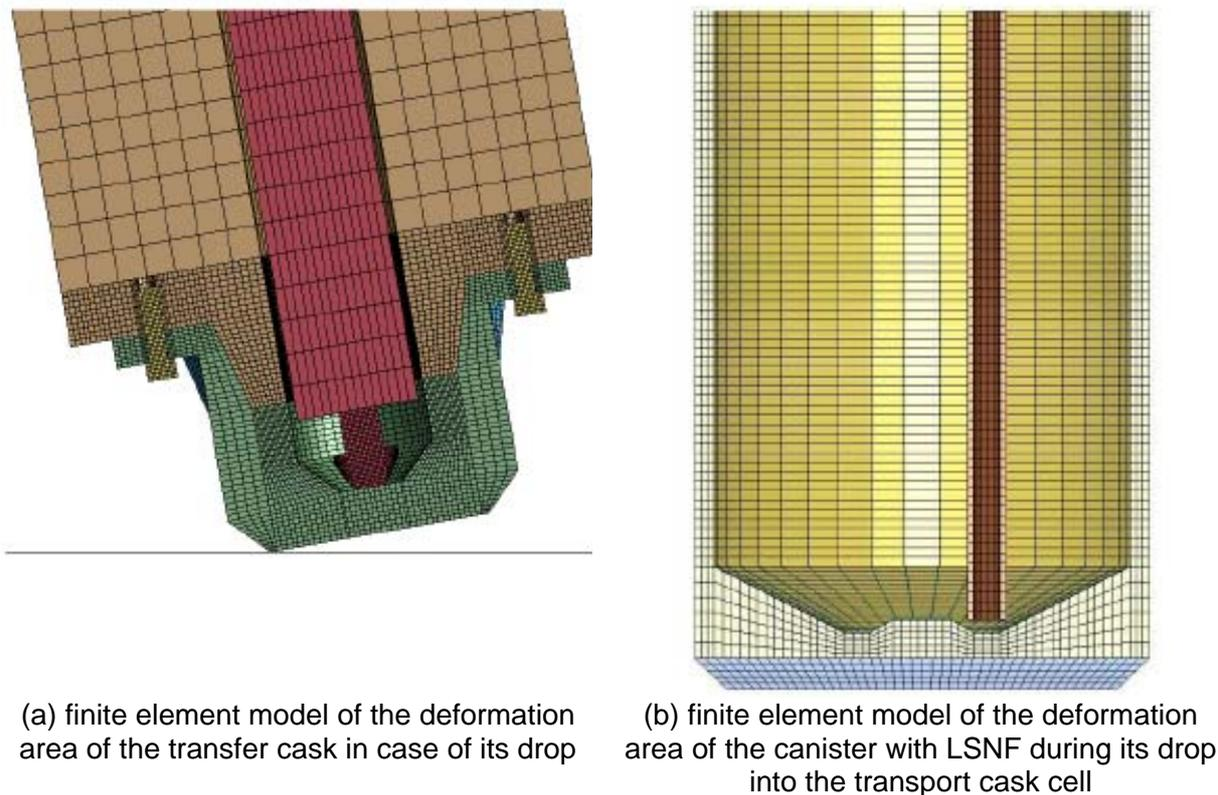
Fig 6. The models used to analyze deformations of the transfer cask and the canister with LSNF after the drop
